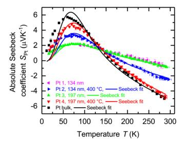
**Above**. Absolute Seebeck coefficient of platinum as a function of the bath temperature *T*. The corresponding solid lines represent the Seebeck fit of the data.
